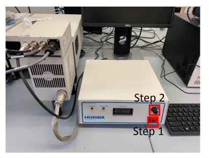
Step1 : Turn on the power supply box by pressing the button
