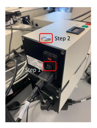
Step 1 Turn on the Power"Power" light indicator is onStep 2 Ignite the lamp"Lamp" light indicator is on
